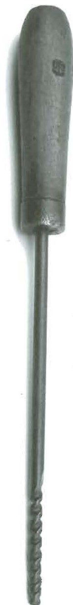
Gunner's gimlet marked with a "US" and anchor, and measuring 12 1/2" long. It was used to bore out obstructions in the vent.
